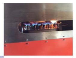
Gas Model adopt import cast iron burner, blue flame, temperature rising fast and stable.
