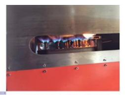
Gas Model adopt import cast iron burner, blue flame, temperature rising fast and stable.
