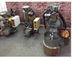
Domestic and Industrial continue roasting design, centrifugal hot air flow circulation with frequency regulation system, roasting temperature is accurate and adjustable.
