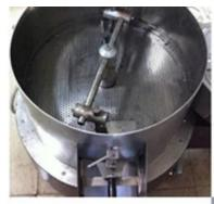
Large cooling tray with high power motor, cooling rapidly within 1-2 minutes, can fasten the coffee flavor
